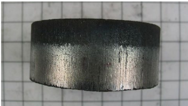
Side profile of HBI produced from ZESTY H 2 -DRI briquetted at 200 MPa, 800 °C (scale: each square is 0.5x0.5 cm)
