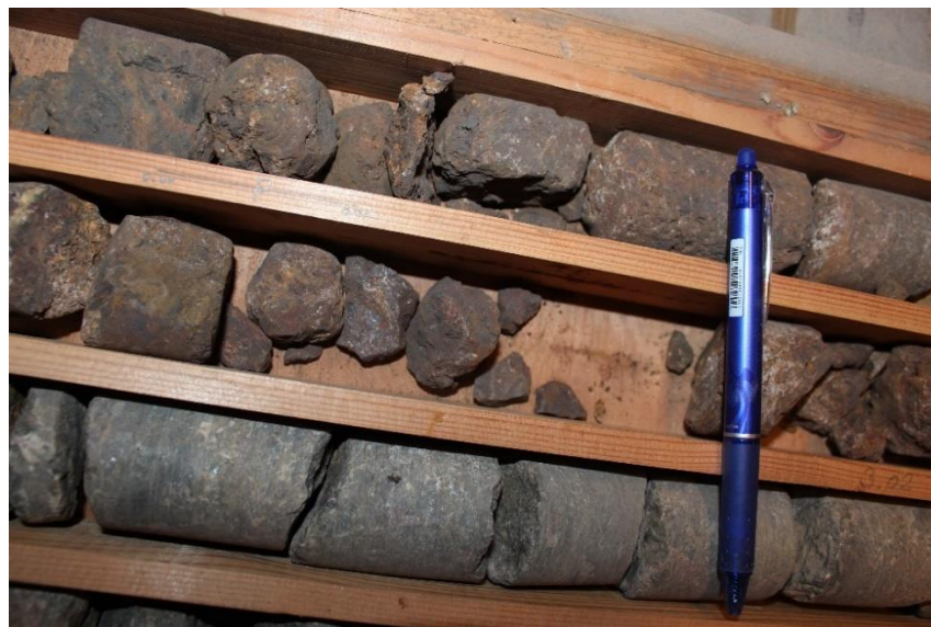
Figure 4: Gronnedal Sample IVT 21 – 4 of carbonatite, and magnetite with 176 parts per million europium (203.8 ppm Eu 2 O 3 ) from 2.8 metres.
