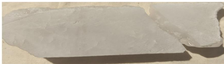
Figure 5: Quartz sample from an Ivigtût prospect that grades 99.7% silica, Sample IVT 21 – 5 from 42.18 metres.
