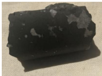
Figure 3: Sample IVT 21 – 1, carbonatite and magnetite from 71.73 metres deep, with 3670 parts per million niobium (5248 ppm Nb 2 O 5 ).
