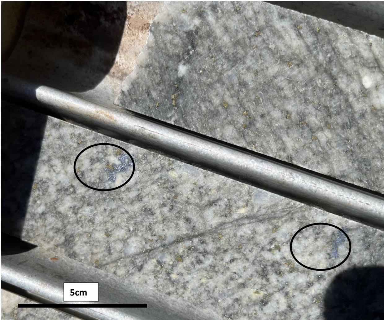
Figure 1 NQ sized diamond core from MSD0002 (149m) 1 drilled by Equatorial Minerals showing blebby molybdenite (silver-grey mineral circled) with disseminated yellowish pyrite in a potassic altered leucogranite. Pyrite is also common in veinlets parallel to the strong foliation and throughout the matrix. Assays by Equatorial Minerals for the interval 148-149m are shown in table 2 below. Details of Minnie Springs historic drilling and assay method and assays > 2,000ppm Mo are listed in Augustus Prospectus Appendix A dated 23 May 2023.
