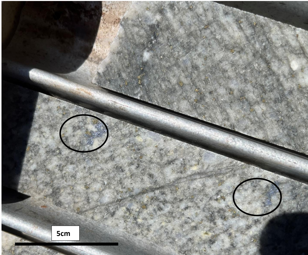
Figure 1 NQ sized diamond core from MSD-2 (150m) drilled by Equatorial Minerals showing blebby molybdenite (silver-grey mineral circled) with disseminated yellowish pyrite in a potassic altered leucogranite. Pyrite is also common in veinlets parallel to the strong foliation and throughout the matrix.
