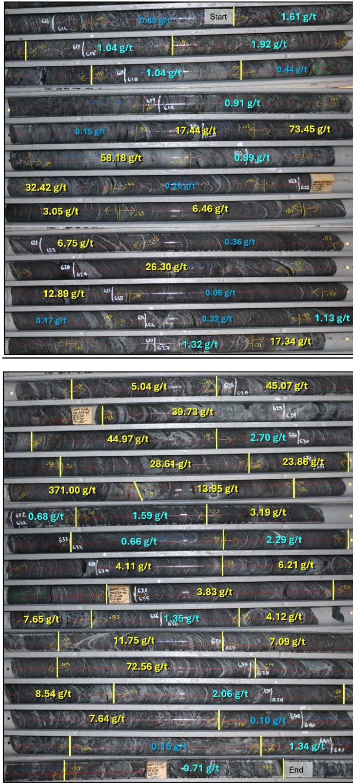
Figure 4: Core photographs of Drillhole DGRC1431-DT-W1 overlaid with gold assay grades from the Pepper Gold Prospect. The mineralised host rock is a metamorphosed and altered, layered, volcanoclastic sequence overprinted with quartz and carbonate veining. "W1" is wedge hole number 1 from parent drill-hole DGRC1431-DT.
