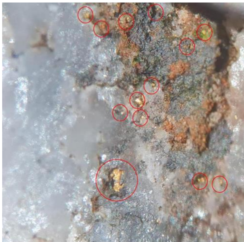
Figure 8: Free Gold in float from quartz reef near the Break of Day Mine
