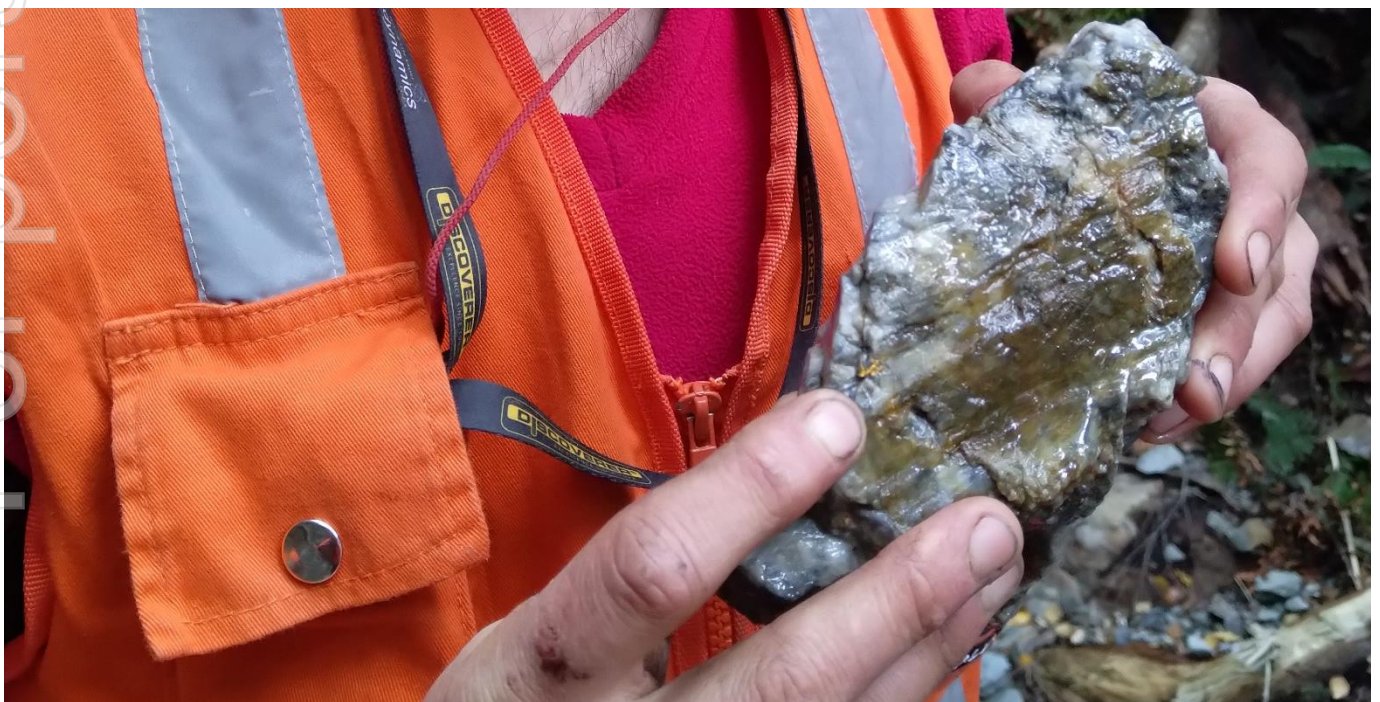
Figure 5: United Victory Reef float sample that assayed 205g/t Au
