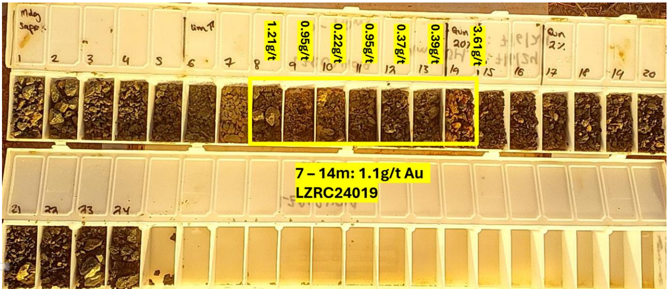
Figure 7 - Chip Tray from LZRC24019 highlighting significant intercept (displayed on Figure 4 cross section B-B' (Figure 2))
