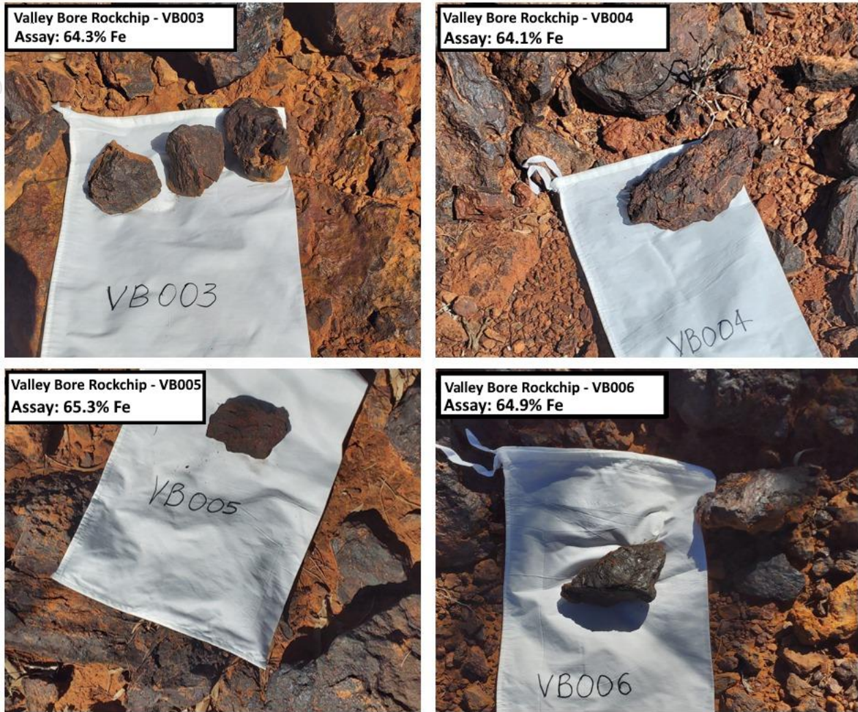
Figure 7: Rock-chip samples with assay results from Valley Bore Southern Ridge target (results in % Fe)
