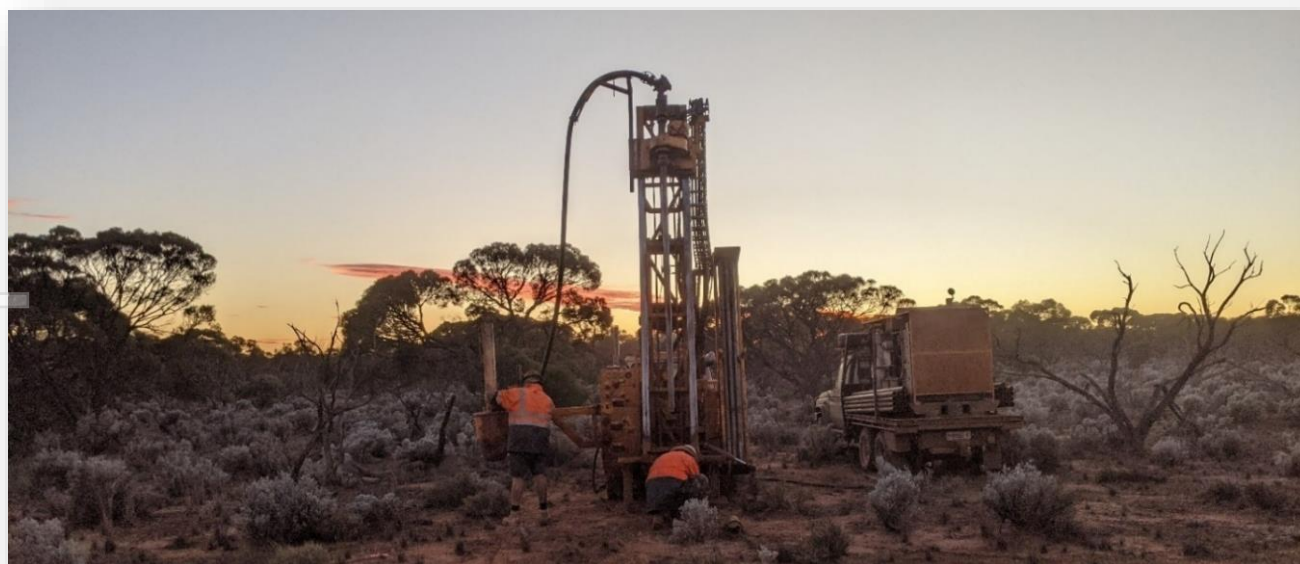
Air-Core drilling at Diomedes prospect during Peterlumbo regional exploration program, March 2024
