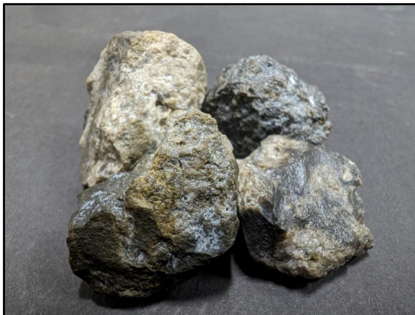
Figure 4. Air-Core chips from the mineralised interval at m 38m in hole PLAC161.
