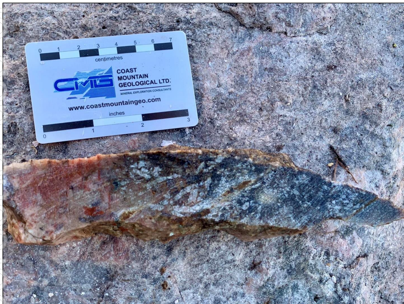
Figure 3 – Medium to fine-grained spodumene within channel sample of the Pegmatite 20 extension
