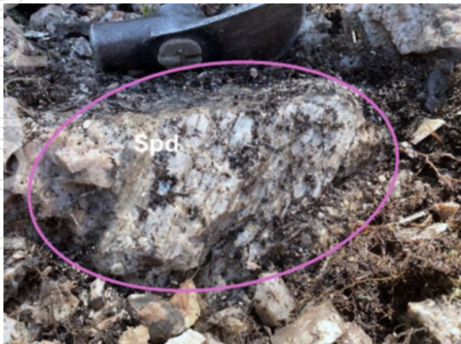
Figure 5 – Left image: very coarse spodumene (Spd) laths up to 30cm in length. Right image: flat lying outcrop, hosting coarse spodumene as distinct from Quartz (Qtz) 1 .
