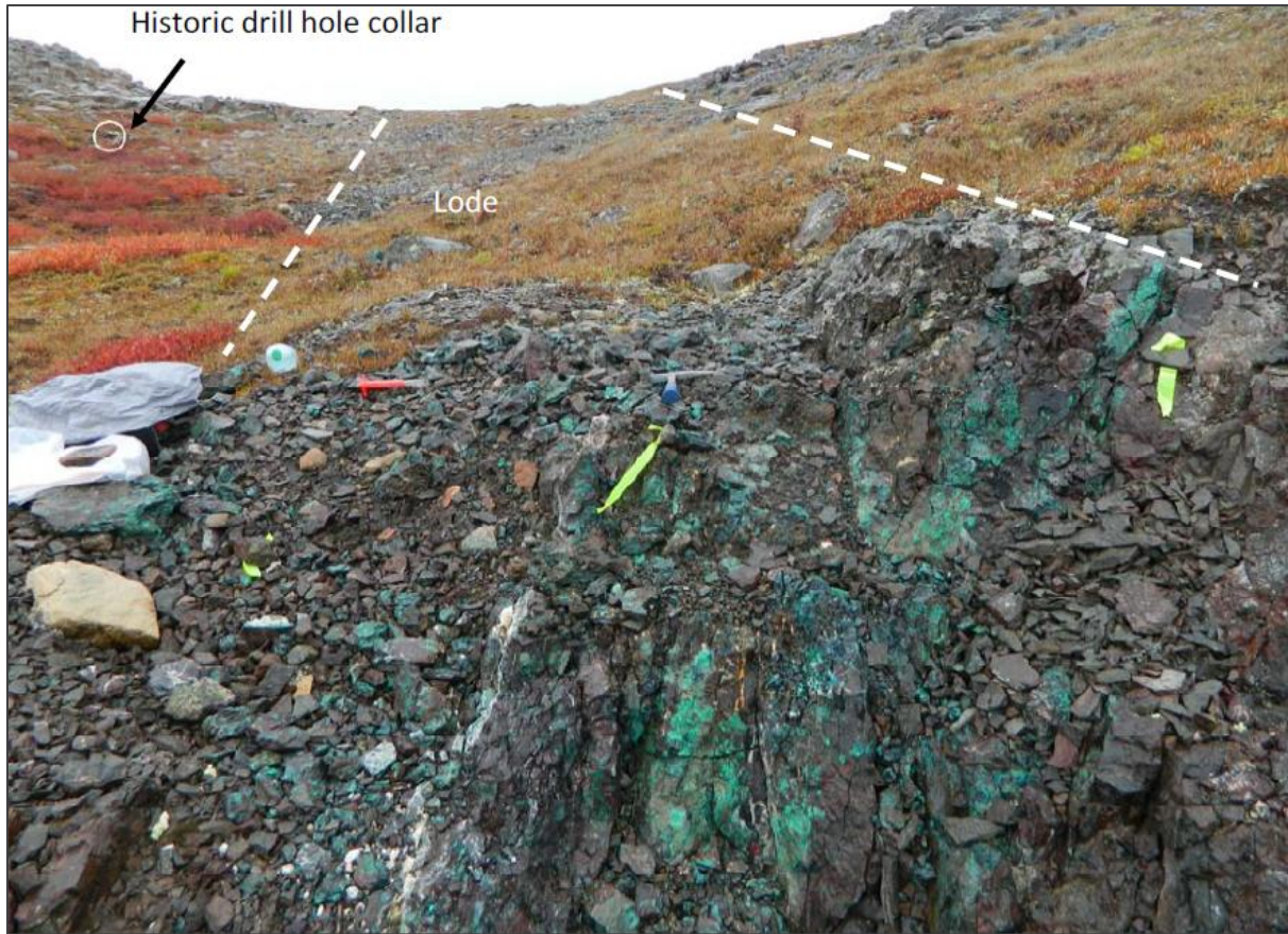
Figure 1 - Field photographs of the Cu-TAR mineralisation (Lode No. 2) taken by Tundra Copper Corp in 2014. Photo illustrates the 2.5 m continuous chip sample which returned 2.5m at 10.3% Cu and 5g/t Ag. (NUMIN File Reference 086024)
