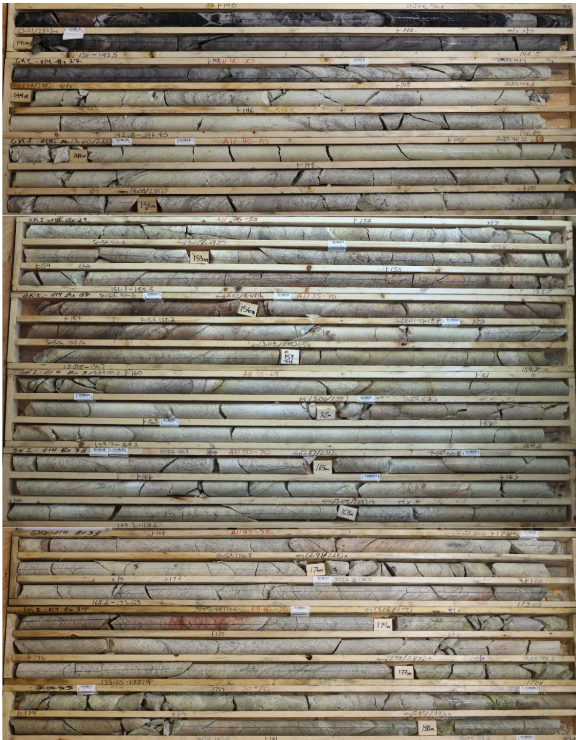
Figure 3: Core photographs showing intense clay alteration in GKI-014.
