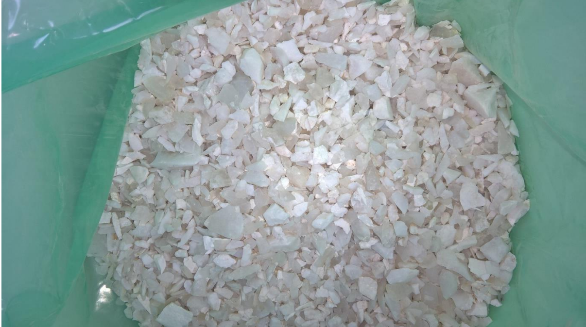
Figure 2: Preliminary products from previous testing work by Jericho Resources Pty Ltd contracted by Rum Jungle Resources Limited in 2016, 99.984% SiO 2
