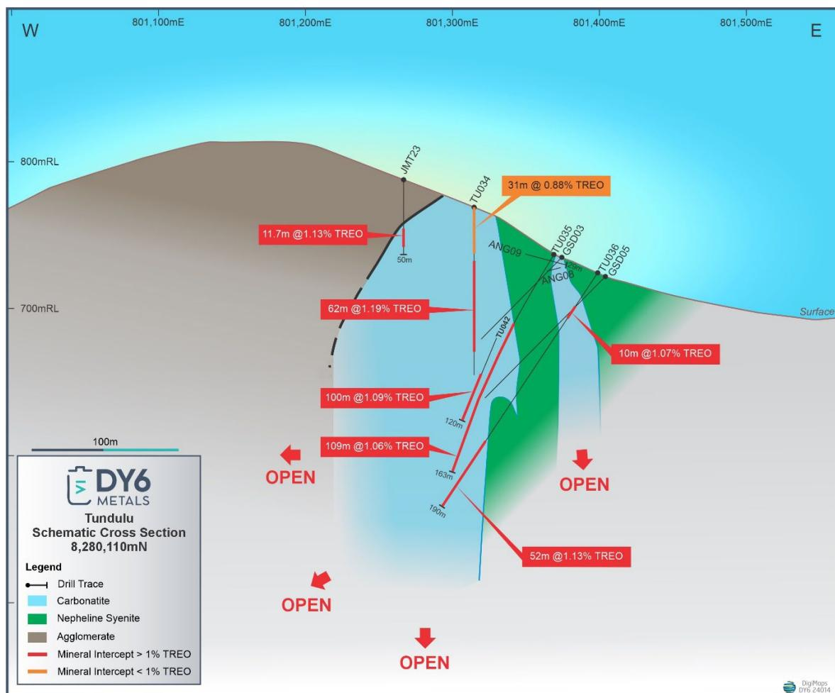
**Figure 9. Schematic Drill Section on 8280115mN +/-15m.**
