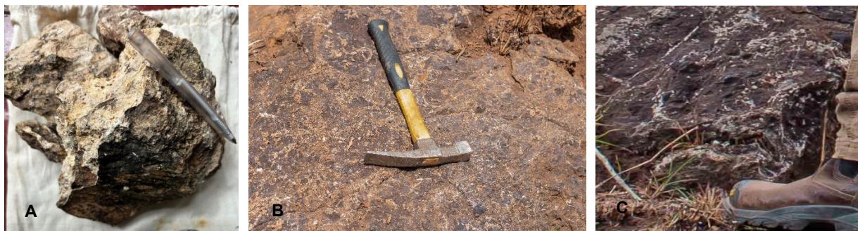
Figure 5. High grade samples Tundu 1 (1.8 wt.% TREO brecciated fenite) (A), BC1 (1.78wt% TREO brecciated carbonatite) (B), BC2B (2.56 wt% TREO carbonatite) (C)
