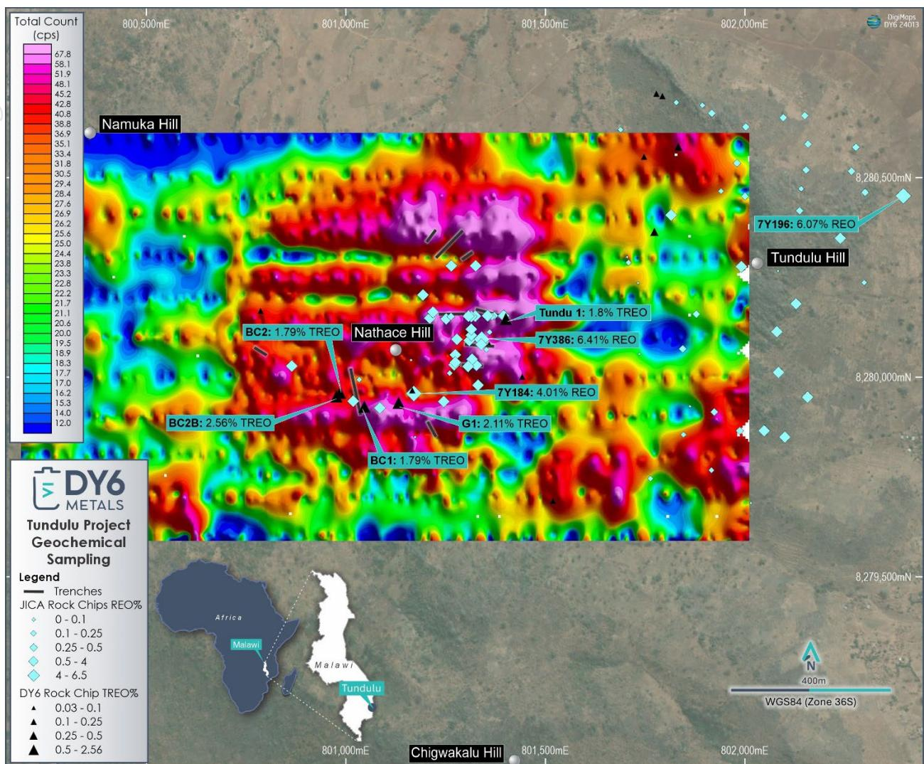
**Figure 10. Ground Radiometric Survey of Tundulu Total Counts/sec**
