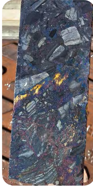
Examples of mineralisation in MOXD 217, 248.9-250m – 1.1m @ 24.8%Cu, 93.2 g/t Ag, 0.11% Co. Bornite, covellite, chalcocite and pyrite matrix fill hydrothermal breccia from within the broader intercept of 66.50m (48.00m estimated true width) @ 4.95% Cu, 32.7 g/t Ag and 685 ppm Co from 234.00m 7
