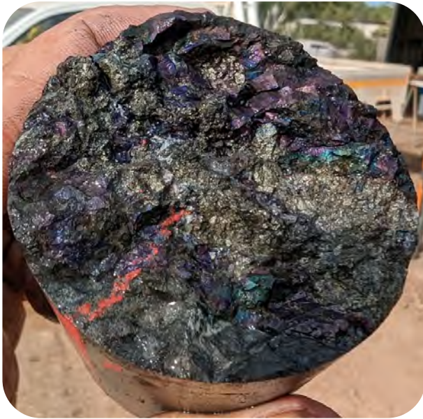
Examples of mineralisation in MOXD 217, 248.9-250m – 1.1m @ 24.8%Cu, 93.2 g/t Ag, 0.11% Co. Bornite, covellite, chalcocite and pyrite matrix fill hydrothermal breccia from within the broader intercept of 66.50m (48.00m estimated true width) @ 4.95% Cu, 32.7 g/t Ag and 685 ppm Co from 234.00m 7
