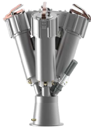
Images: The plasma torch used in Turquoise Group's process (L), and graphene powder generated through the trial demonstration (R).
