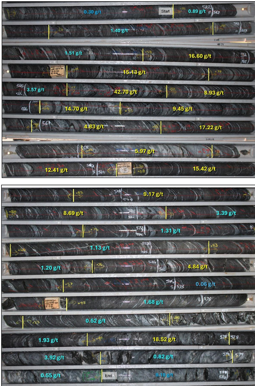
Figure 4: Core photographs of Drillhole DGDH069W1 overlaid with gold assay grades from the Pepper Gold Prospect. “W1” stands for wedge hole number 1 from parent drillhole DGDH069.
