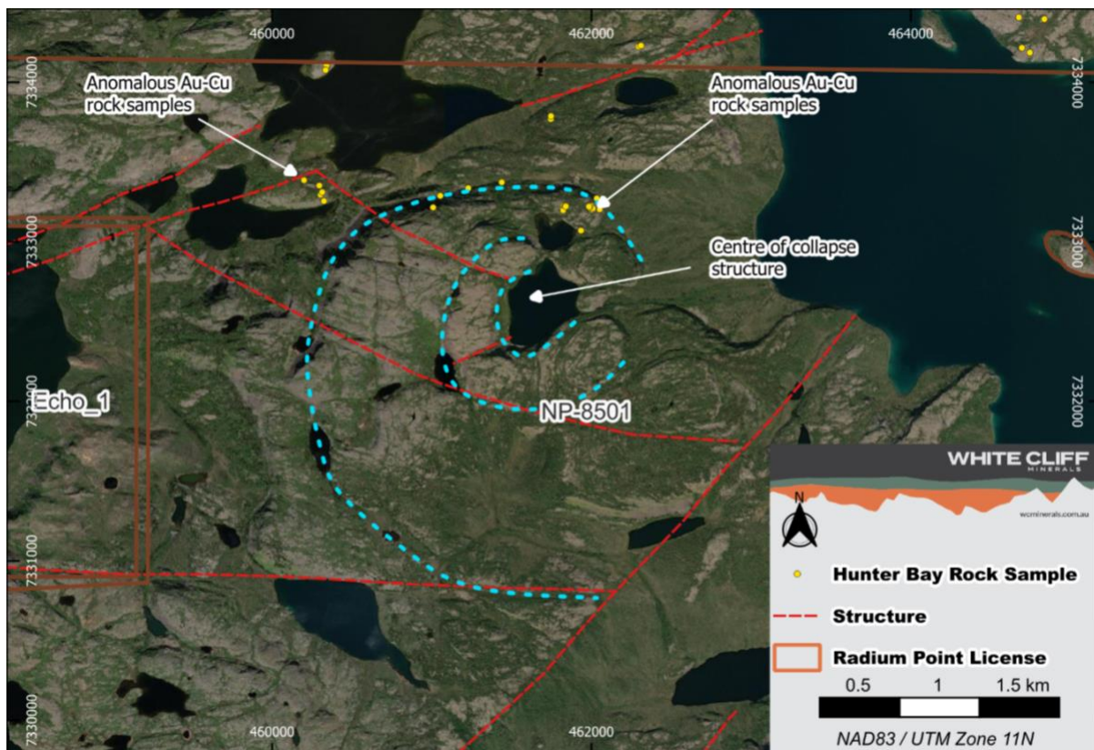
Figure 3 - Map of the Sparkplug Lake target area. Anomalous Au-Cu rock chip samples taken immediately north of a clear collapse feature with an annular appearance in satellite imagery. Several fault orientations are observed with mineralisation associated with a major ENE/WSW structure.
