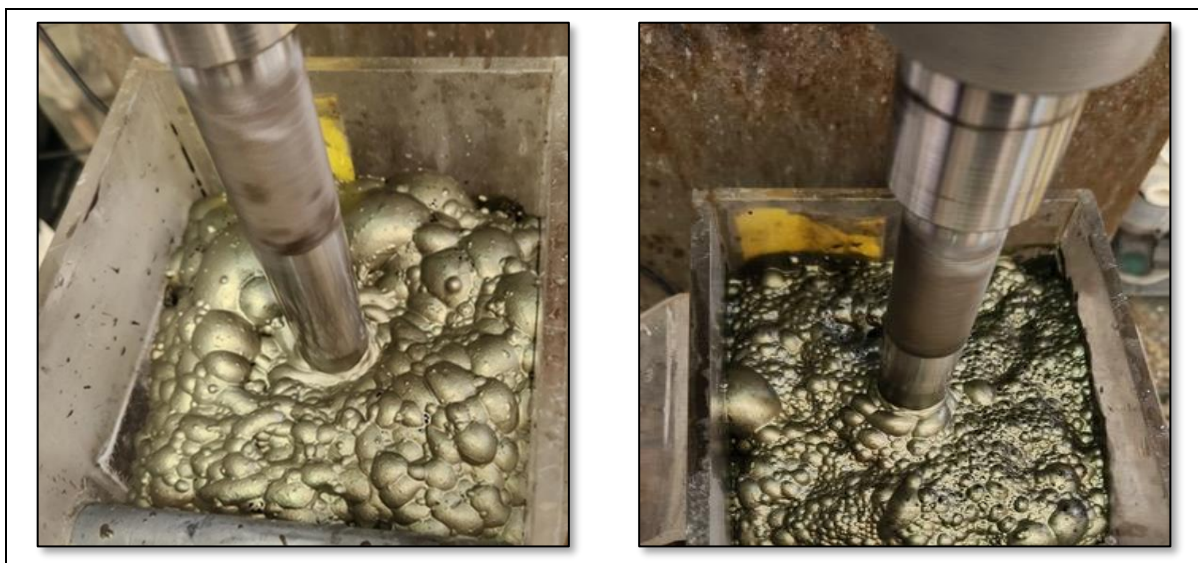
Figure 1: Cleaner Flotation Concentration of Chalcopyrite from BBDD0045, Bluebird Copper-Gold Discovery
