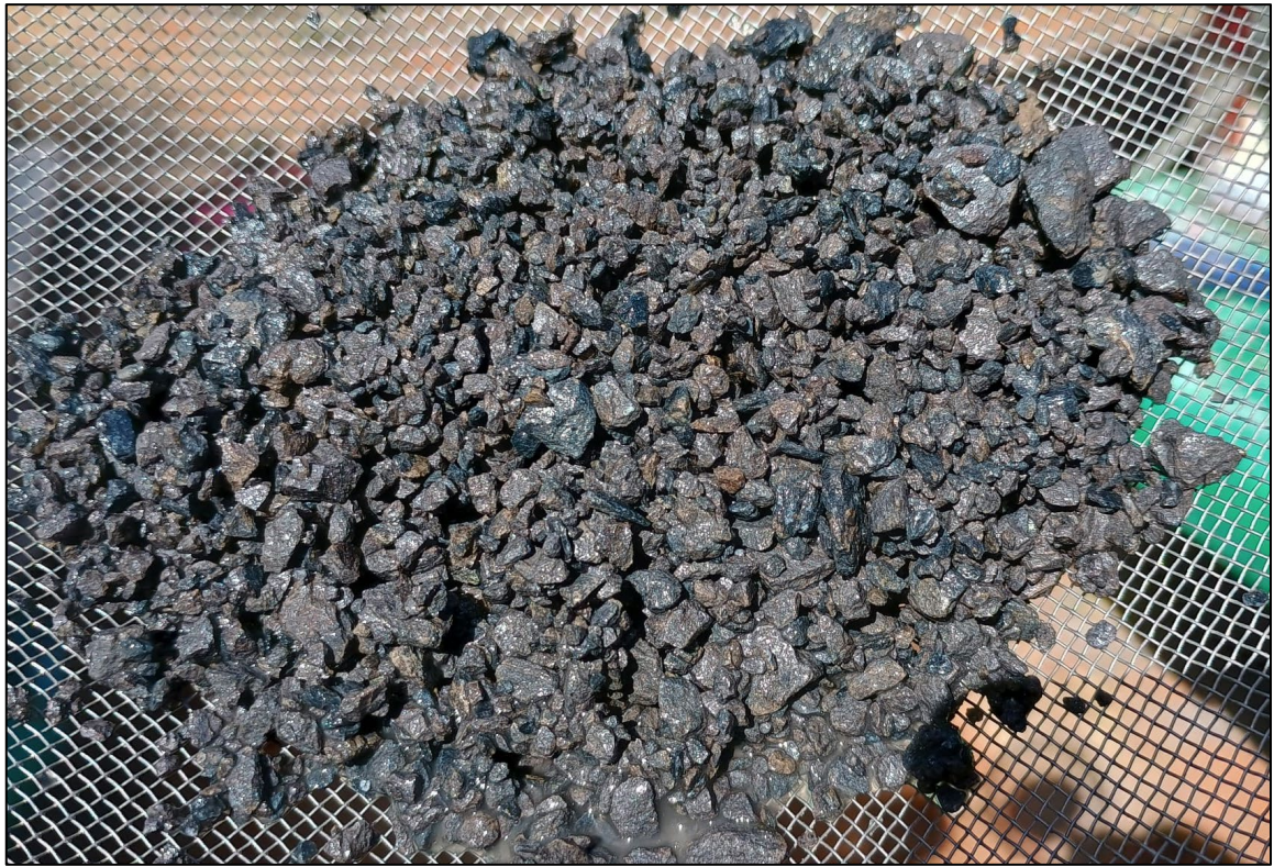
Figure 1: A3RC030 photo of massive sulphide from 115-116m, comprising the zinc mineral sphalerite (brown) and lead mineral galena (grey). This exceptionally high-grade interval yielded 13.8g/t gold, at least 3,000g/t silver, 11.4% lead and 27.4% zinc.
