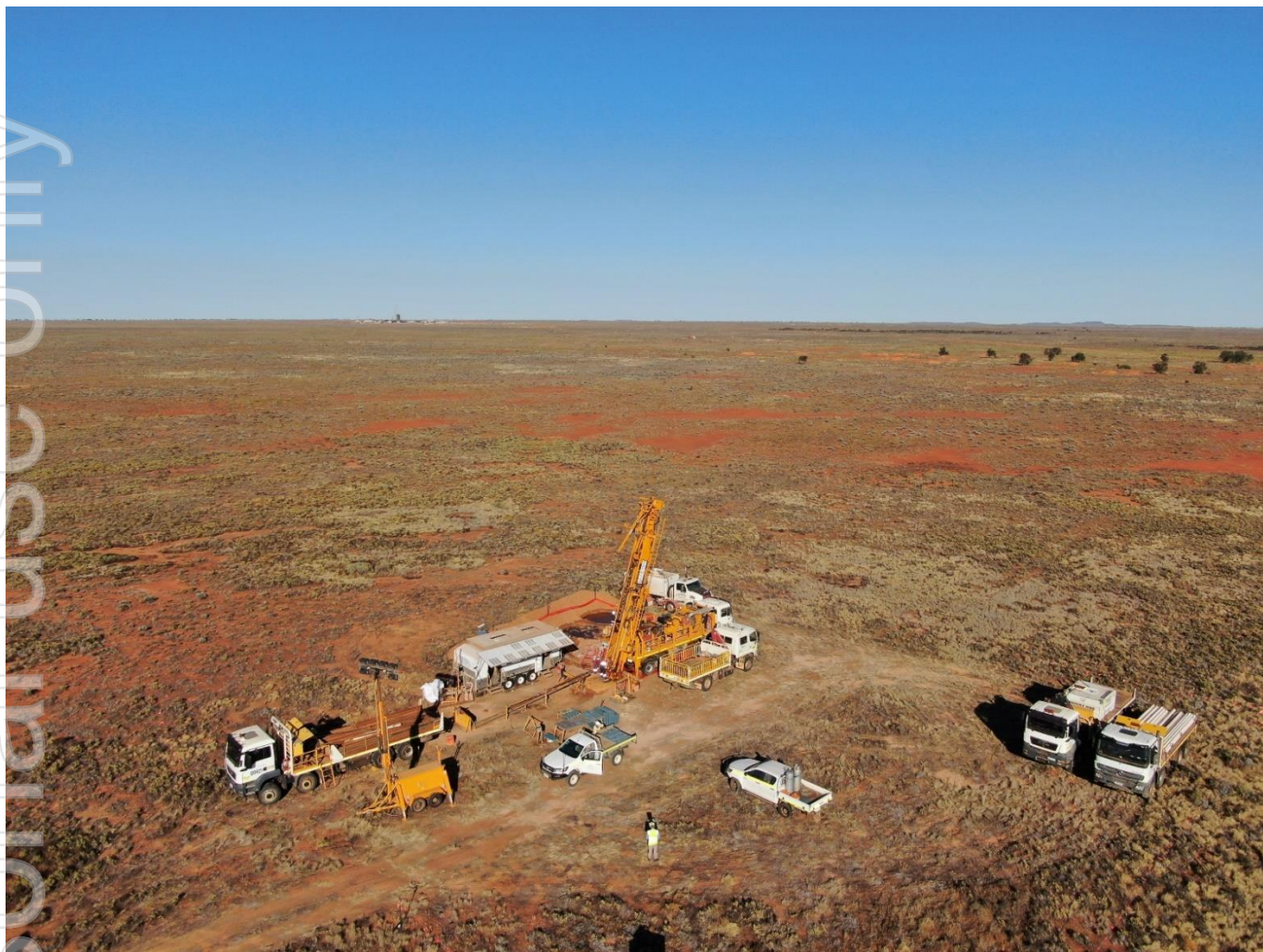
Figure 3: Diamond drilling at Atlas target, 4km east of Honeymoon mine
