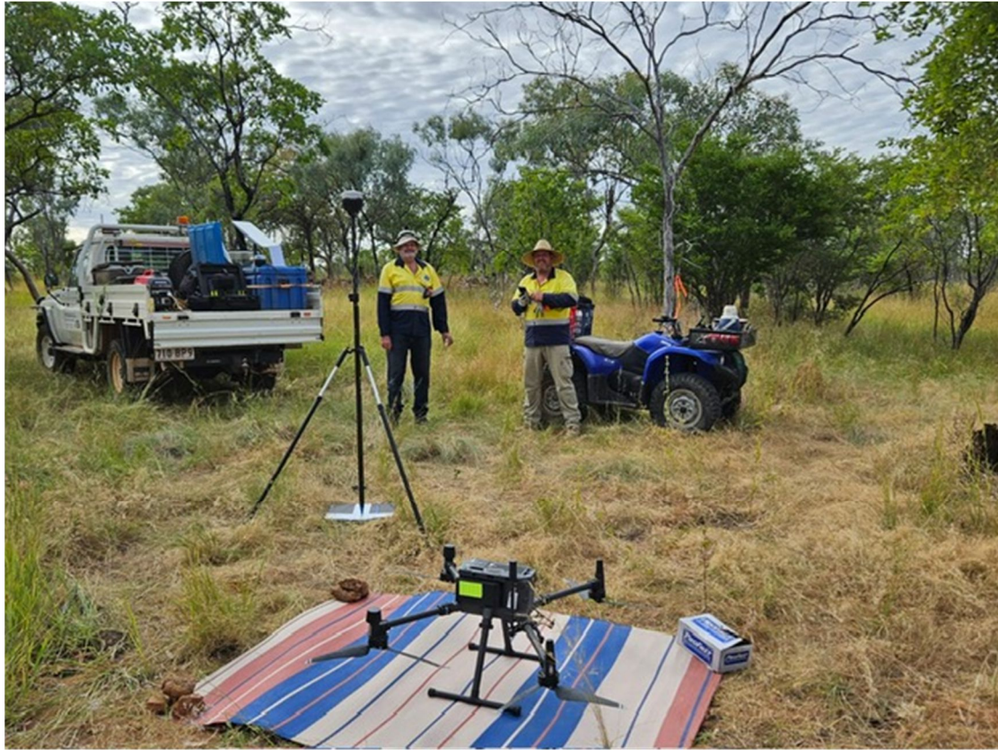
Figure 4. Drone LIDAR, Photogrammetry Survey station at Fiery Creek Copper prospect
