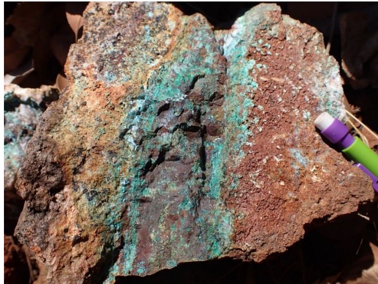
Figure 2. Sample ESL 2588. A high-grade oxide copper (cuprite, tenorite, malachite and chrysocolla) vein from the Eastern Shear Zone hosted quartz with Cu, Fe oxides and oxyhydroxides, Fiery Creek Copper prospect. (Sample location 774773E, 8007952N)
