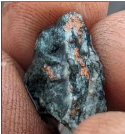
Figure 6. Examples of (left) Native Copper development (scale 2cm) in upper gabbronorite hanging wall; and (right) copper-sulphides (scale 1cm) in the basal Crius Reef
