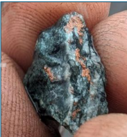
Figure 6. Examples of (left) Native Copper development (scale 2cm) in upper gabbronorite hanging wall; and (right) copper-sulphides (scale 1cm) in the basal Crius Reef
