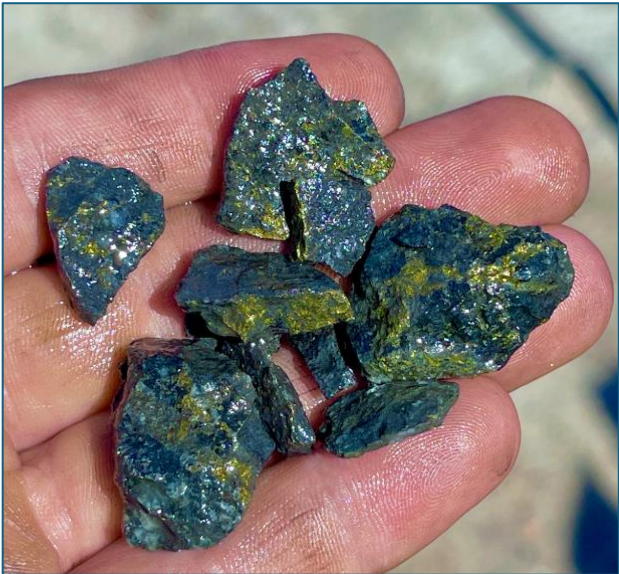
Figure 1. Magmatic sulphide mineralisation in CRC003 (80-81m) grading 0.94% Cu.
