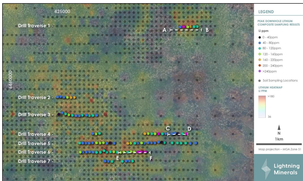
Figure 2: Peak downhole lithium result plan for composite samples within E63/2000 Aircore program. (Background lithium heatmap derived from UFF+ lithium soil geochemistry results)
