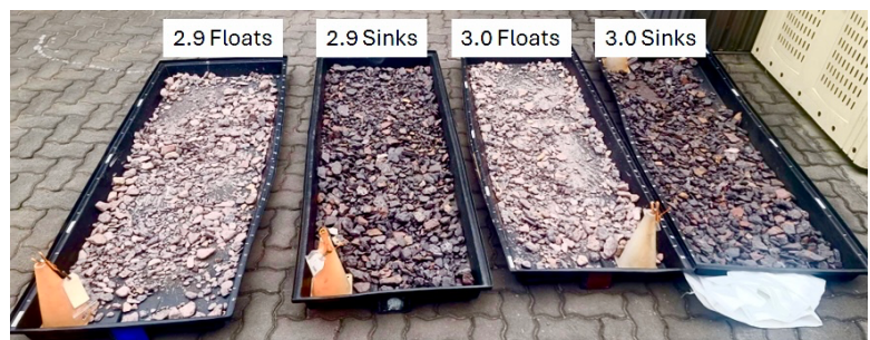
Figure 3. DMS testwork sample trays showing sinks (dark) and floats (light).
