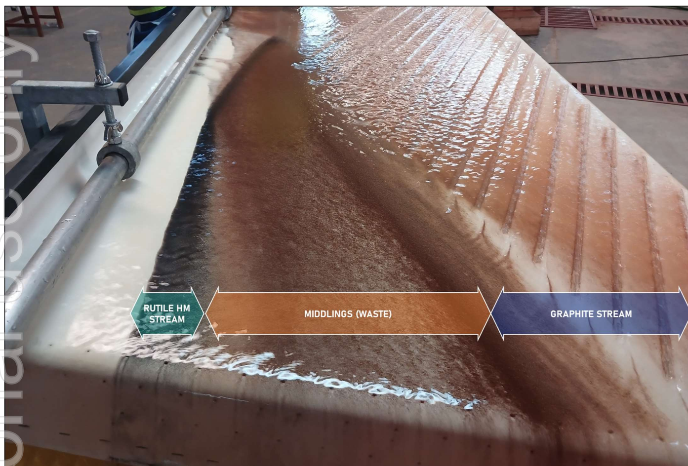
Figure 1: Holman Wilfley 2000 wet shaking table in action demonstrating clear separation between Rutile HM, waste and Graphite
