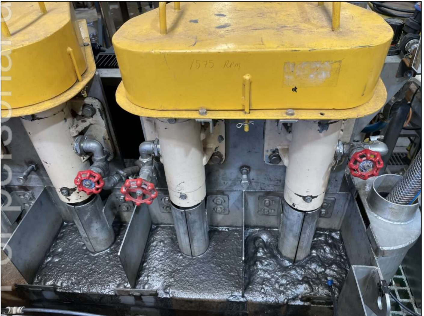
Figure 2: Graphite flotation test work at Australia-based ALS Global
