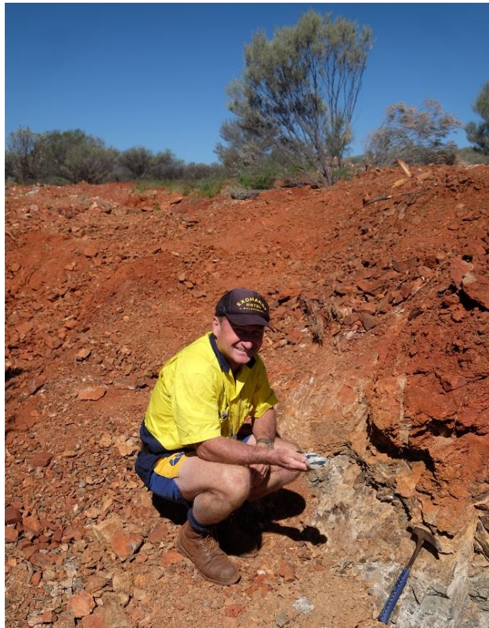
Figure 3: Icen Gold Managing Director Wade Johnson inspecting the recently exposed geology within the sample pit and collecting information on the orientation and nature of the gold bearing shear zone and veinlets. Photo looking towards the southeast.
