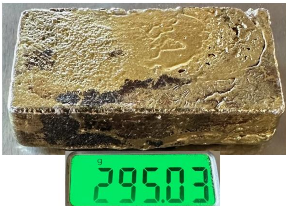
Figure 6 ~9.5oz gold doré bar* poured by the prospectors, produced from 101.3kg of Christmas Gift ore samples with a calculated grade of 2,912.4g/t**.
