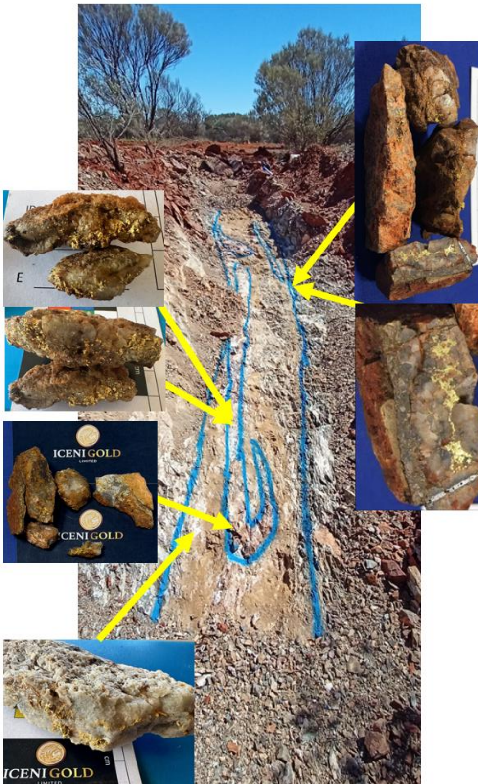
Figure 2: Recently exposed sample trench that has greatly enhanced the visibility of the Christmas Gift structure, which contains the quartz gold* veinlets. Approximate location of gold recovered from the mineralised zone*; Left side photos are newly discovered gold bearing veins, while right side photos are taken from ASX release of 8 June 2023. Photo looking northwest (bearing 310 degrees) along the strike of the structure.
