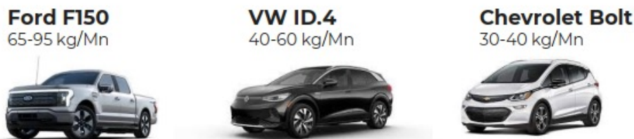
Figure 17: Mn content (kg) per battery in each vehicle above (Source: Benchmark Mineral Intelligence)
