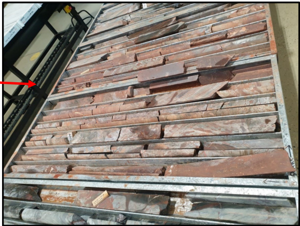
Zone of strong hematite IOCG style alteration (rust red colouration) in hole ABNE 2 (interval 417.9m – 426 m)
