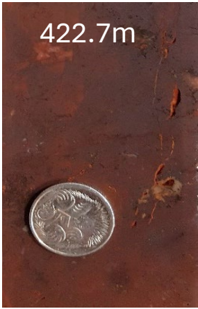
Zone of strong hematite IOCG style alteration (rust red colouration) in hole ABNE 2 (interval 417.9m – 426 m)
