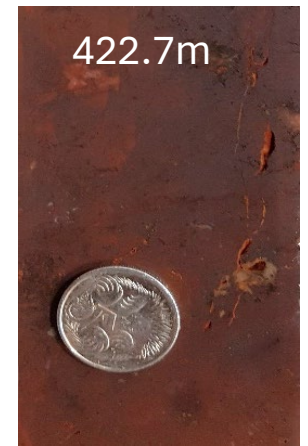
Zone of strong hematite IOCG style alteration (rust red colouration) in hole ABNE 2 (interval 417.9m – 426 m)
