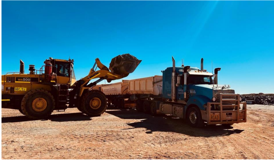
Figure 1 - ROM Loader placing Second Fortune gold ore into road train (April 2024)
