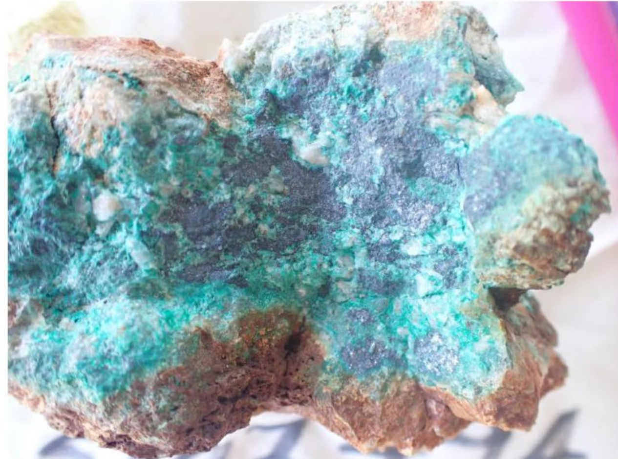
Sample ESSO2494 – (460ppm Ag, 1.25% Ba, 23.51% Cu, 14ppm In). White frosty quartz vein invaded by a later massive sulphide event as a mix of black tenorite ( \text{CuO} ) and sooty to dark grey chalcocite ( \text{Cu}_2\text{S} ) replaced at its margins by crystalline fibrous malachite and minor chrysocolla (Coordinates Location 773511E 8007365N).
