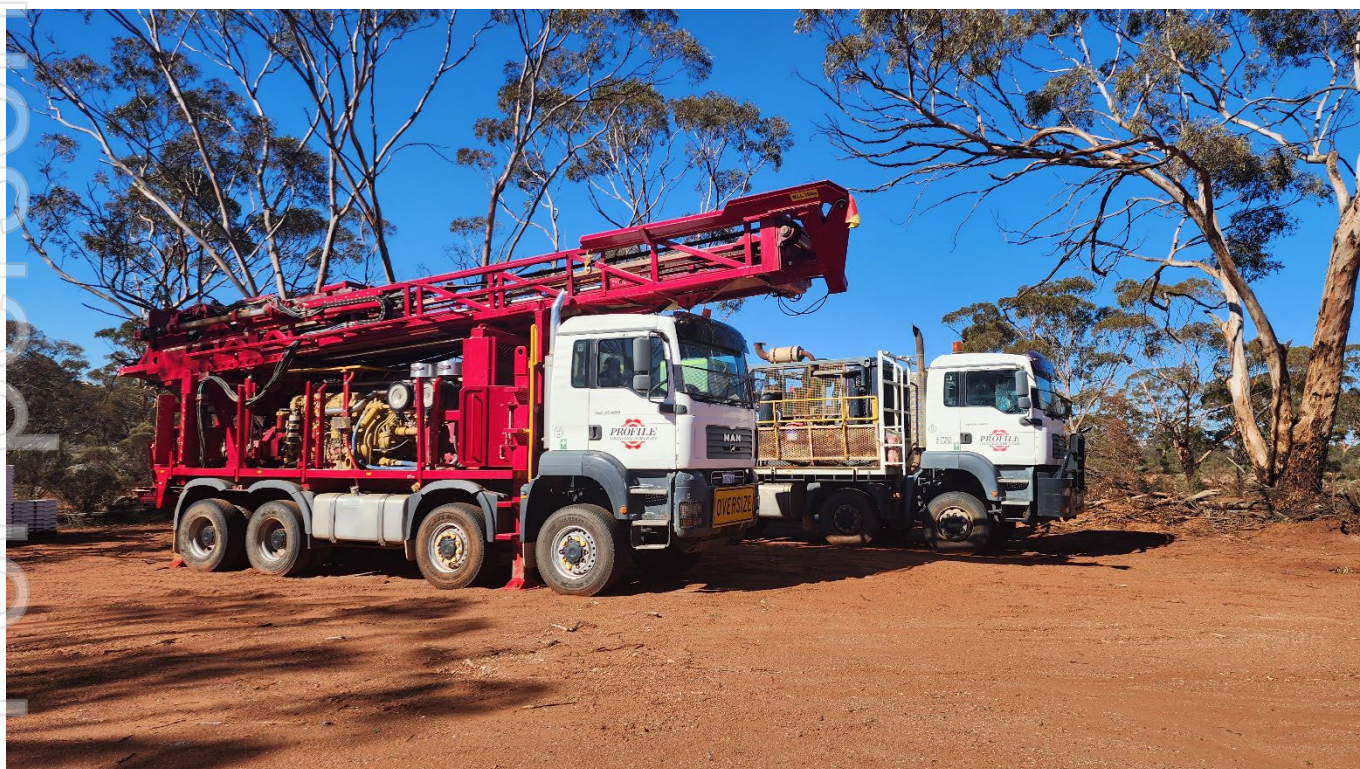
Figure 3. Profile RC rig on site at the Manna Lithium Project.
