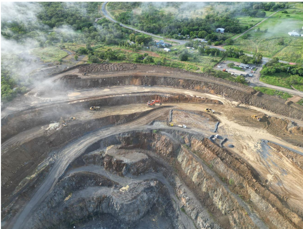
Picture above: Stripping ongoing with the noise and visual bund construction progression.
