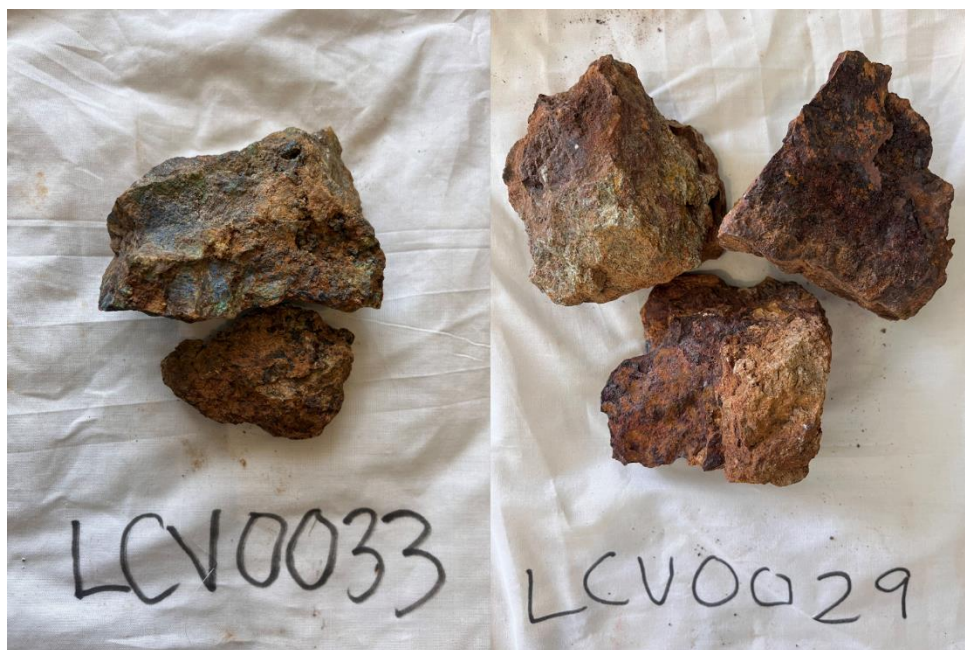
Figure 4 - Example of gold, copper and silver mineralised sample from Long Tunnel area (left) and to the SSE near but not at the Happy Days prospect (right).
