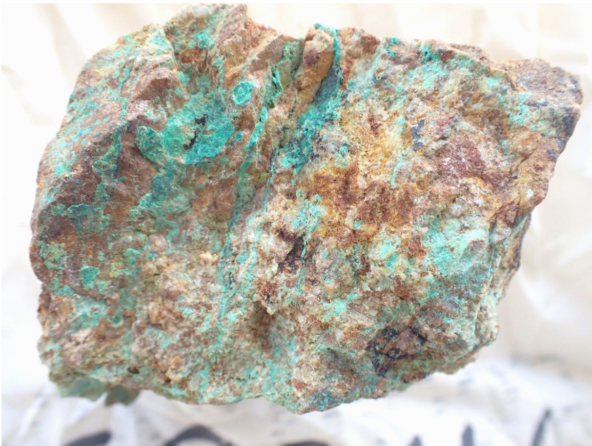
Figure 4: Sample ESSO 2116. (63ppm Ag, 815ppm Bi, 6.26% Cu, 2090ppm Pb) Intensely weathered and oxidised, quartz (vein and veinlet replacement) + sericite + goethite + limonite + chrysocolla + malachite altered granodiorite with secondary drusy cavities infilled with late-stage prismatic quartz.
