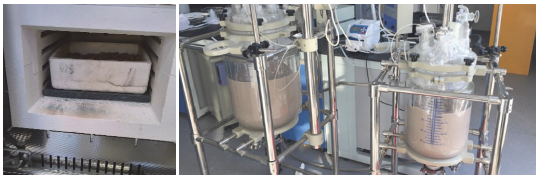
Sulphation Roasting (Left) and Leaching (Right)
