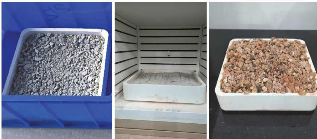
Calcination of Spodumene – Before and After
