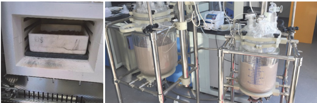
Sulphation Roasting (Left) and Leaching (Right)
