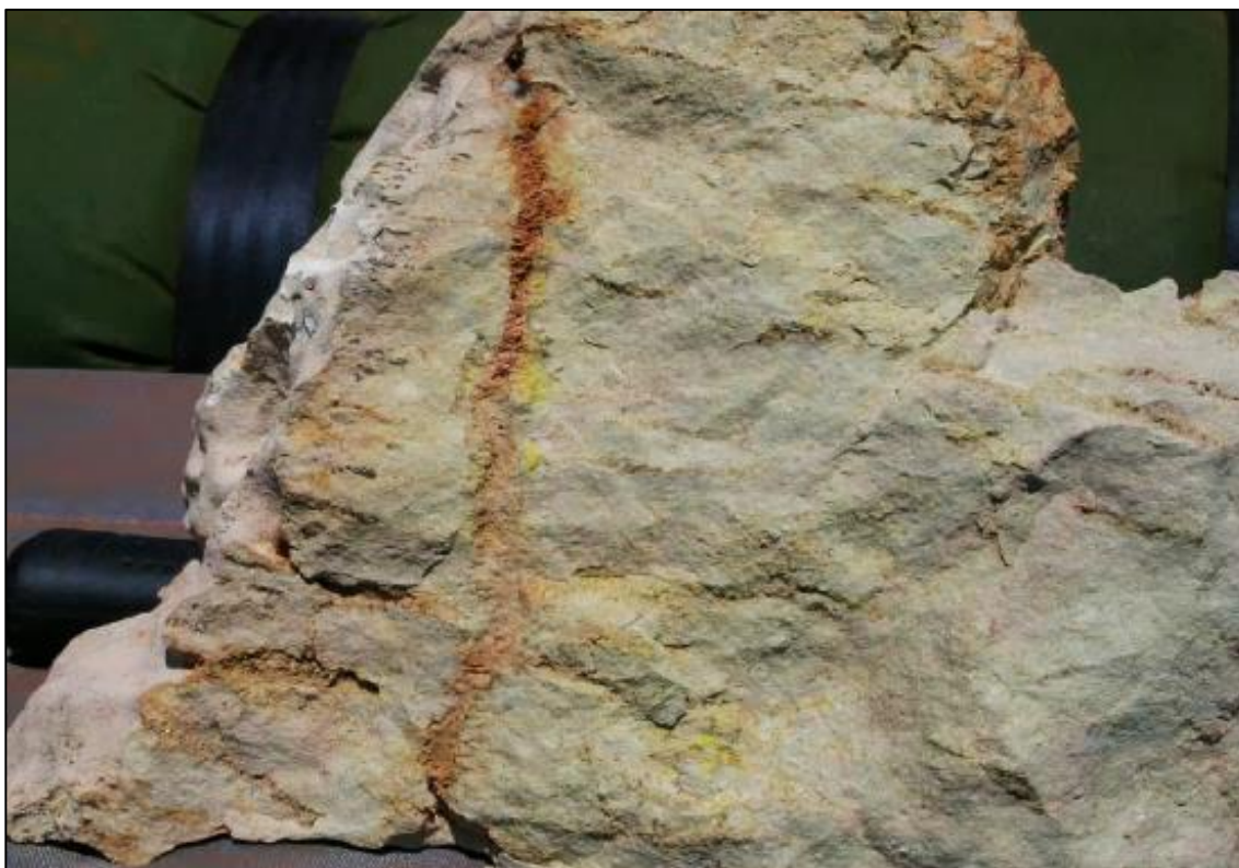
Figure 3: Carnotite (uranium) mineralisation (yellow mineral) in porous sandy limestone from the Ben Hur prospect.
