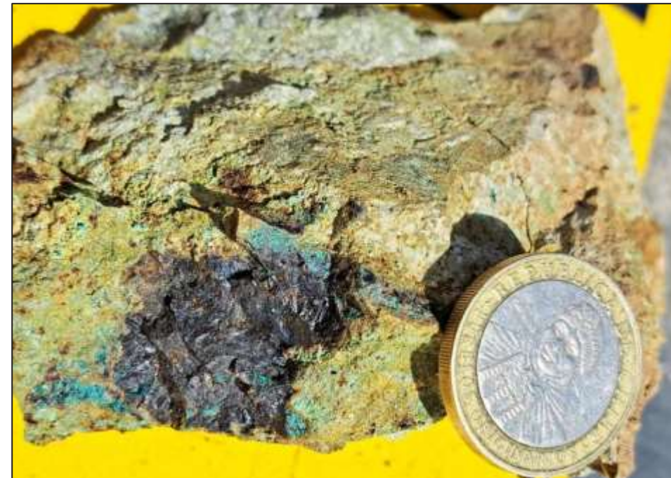
Sample # 8615 grading 5.37% Cu from the Lucero Prospect 2 .
