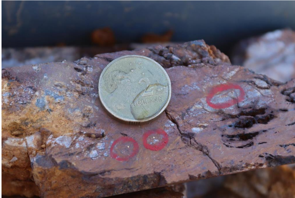
Figure 7 - CTWMET003 at 54.05m, showing visible gold (VG, circled) with $2 coin (20.5mm diameter) for scale
