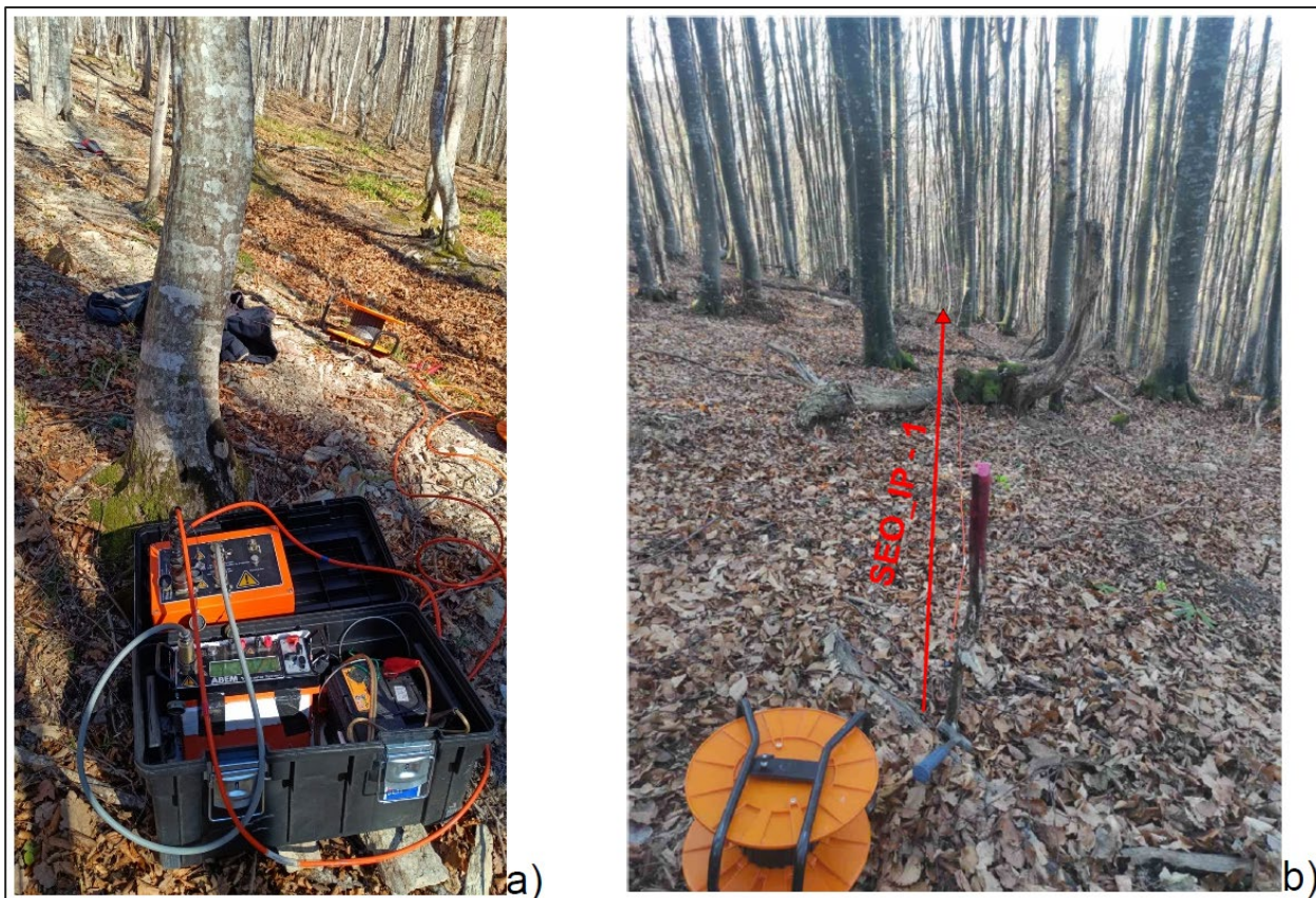
Figure 3: Field photos showing a) ABEM Terrameter System and LUND Imaging electrode selector; and b) survey line start location (labelled A' on Figure 2)
