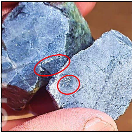
Figure 10: visible gold in cut samples at 123 to 124m interval (above) and sulphide mineralisation in sediments (right) at 123.4m drill depth
