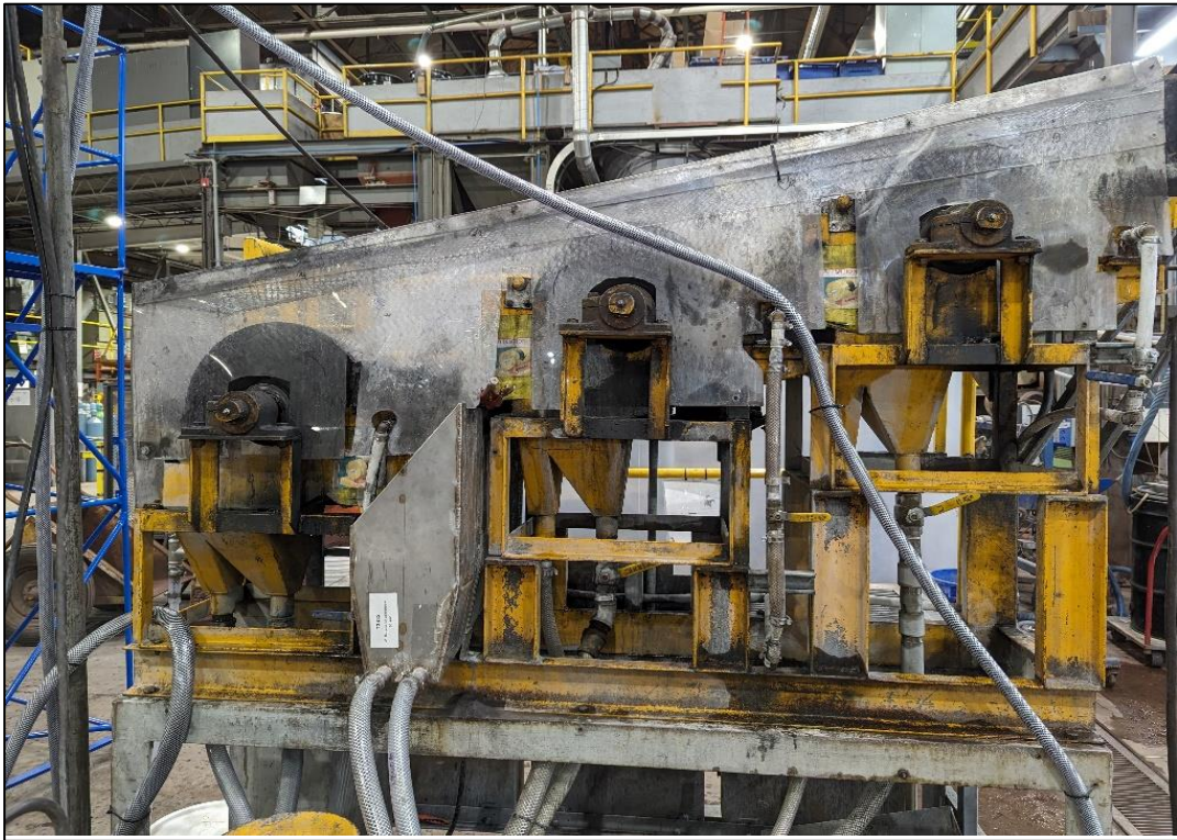
Figure 3: 3-stage WLIMS (Wet Low Intensity Magnetic Separation) industrial unit
