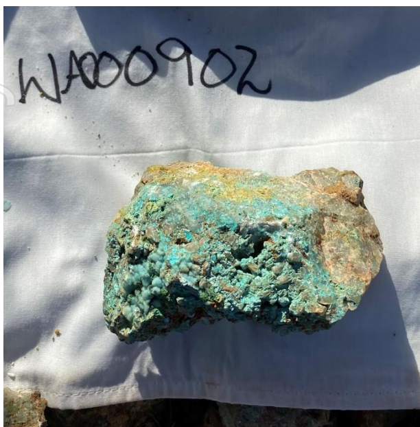
• Copper rich quartz vein assayed 5.6% Cu and 0.43% Pb
