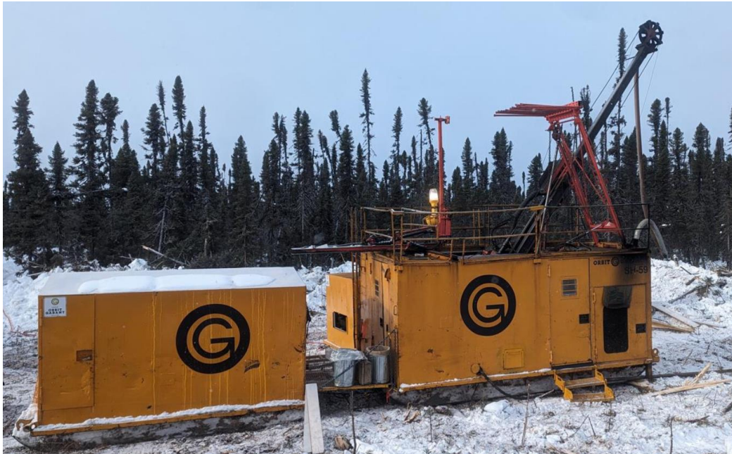
Figure 2: Diamond drill rig at Horden Lake project
