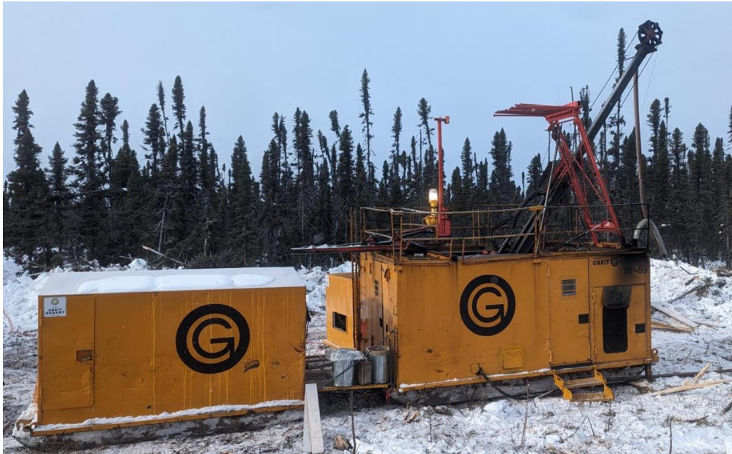
Figure 2: Diamond drill rig at Horden Lake project
