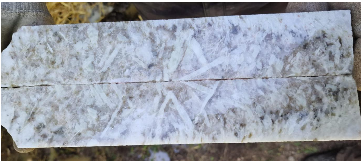
Figure 6: Spodumene pegmatite in drill core DDH 23-1597-01 (PEG-01 [part of]; 34.59-34.94. Sample AES65107 reporting intercept apparent thickness of 0.36m \ True thickness 0.05m @ 2.95% Li 2 O)
