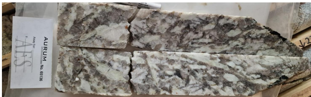
Figure 7: Spodumene pegmatite in drill core DDH 23-1597-02 (PEG-04; 31.46-31.85. Sample AES65136 reporting 0.39m @ 1.59% Li 2 O)
