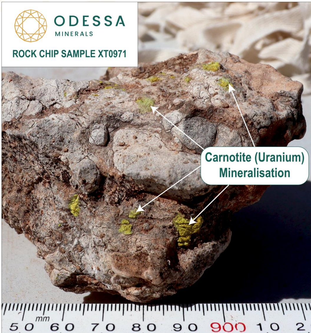
Figure 3: Carnotite (uranium) mineralisation within reworked siliceous calcrete at Baltic Bore in sample XT0971.
