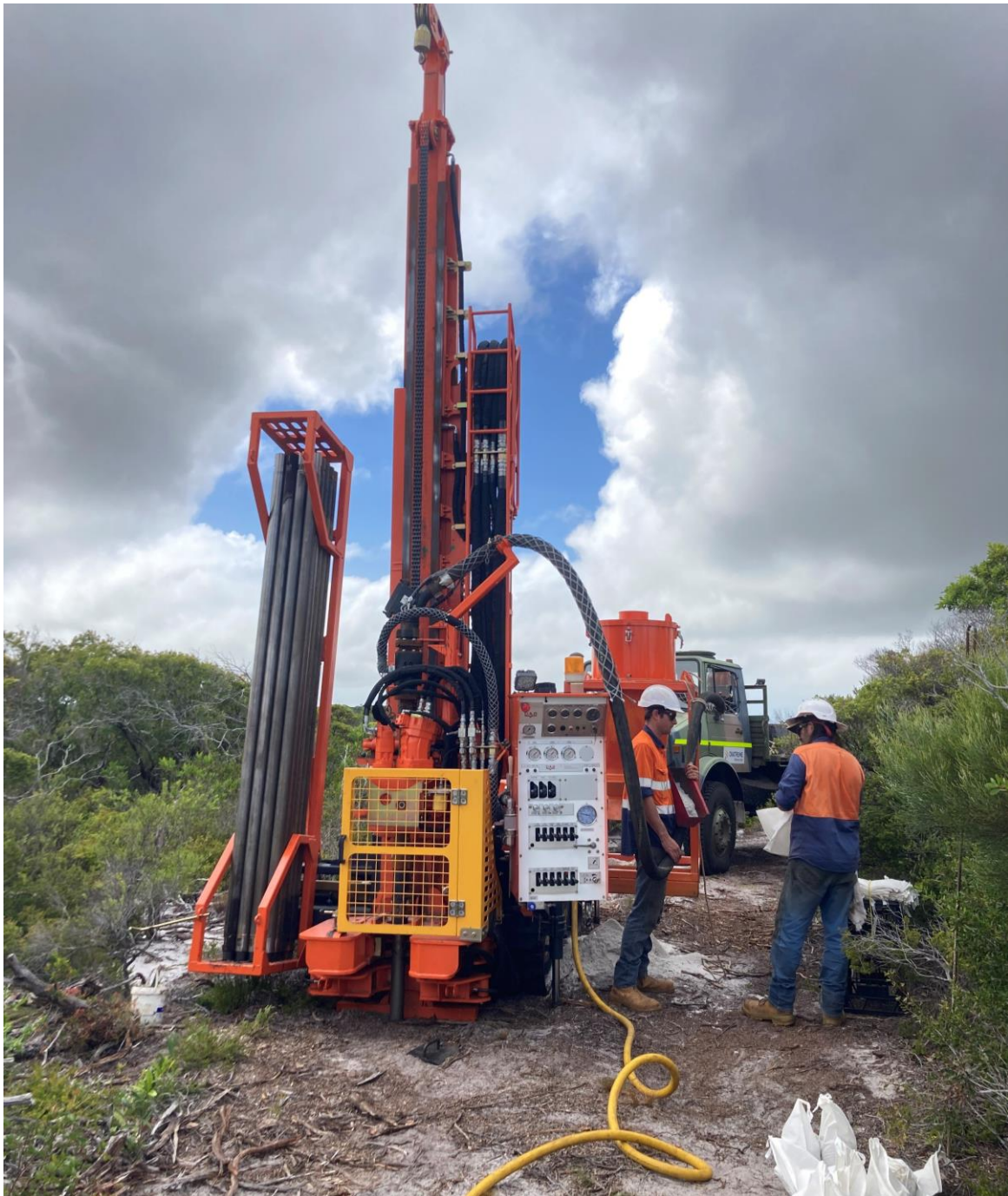
Figure 4: Diatreme Resources' Aircore drill rig showing sub-sample collection after the riffle splitter.
