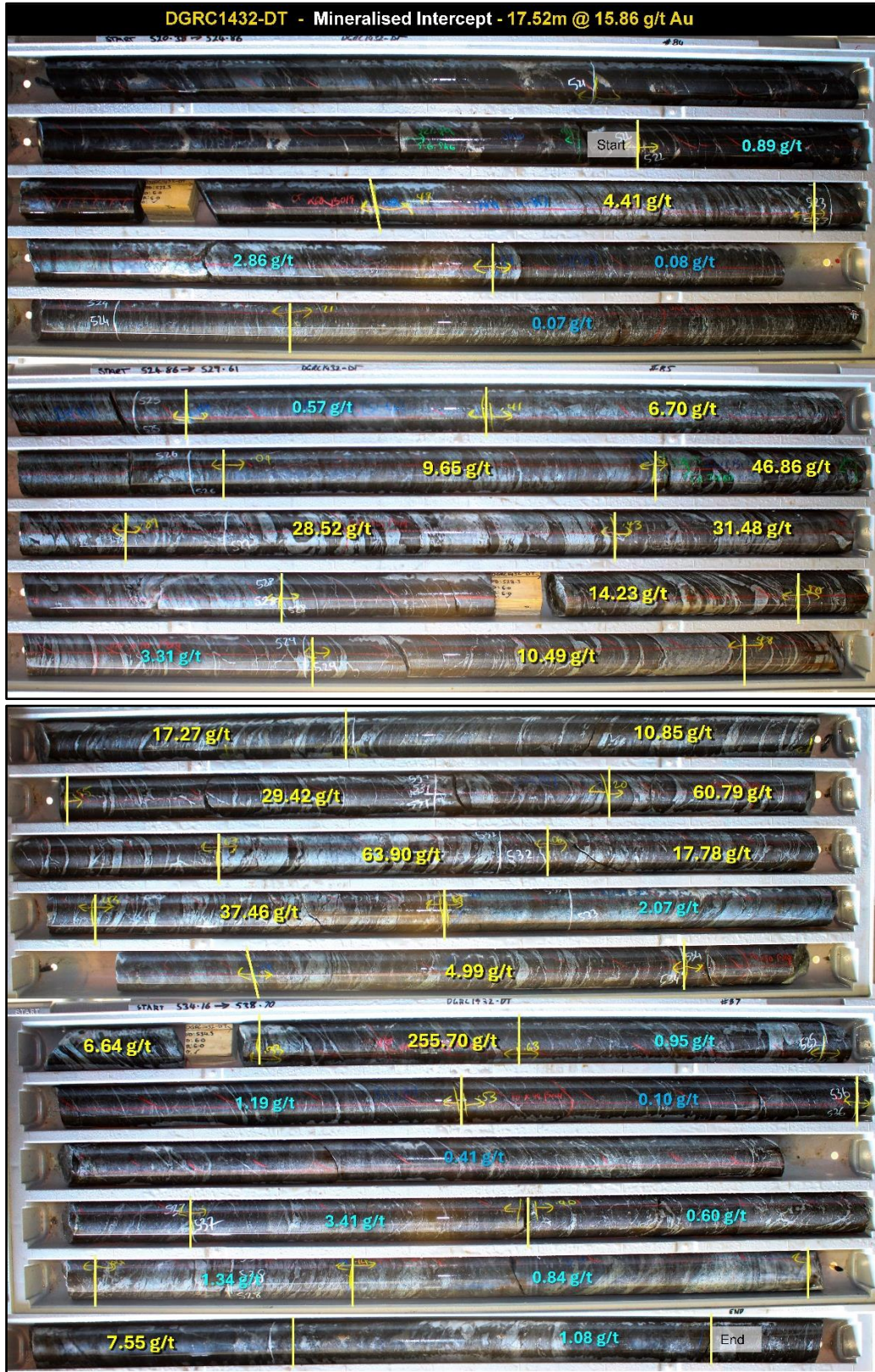
Figure 3: Core tray photographs of DGRC1432-DT "Pepper" discovery hole with gold assays overlaid.
