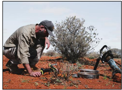
Figure 6: Asra's Exploration Manager at Yttria inspecting drill chips and taking Niton pXRF readings of soil samples.
