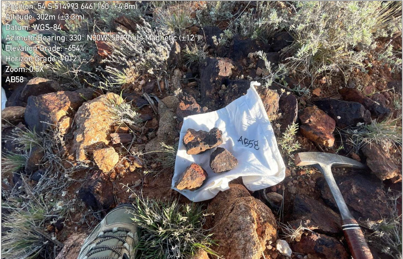
Figure 7: Bald Hill Northeast target – photo of rock chip sample B00605 (gossanous quartz albite gneiss) which assayed 0.18% cobalt and 0.46% copper.
